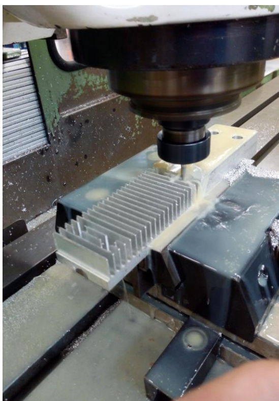
Figure 10: Fins casing manufacturing for the cooling system
