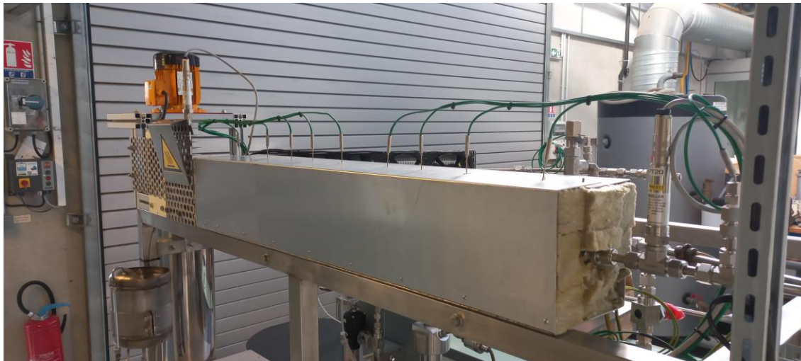
Figure 9: Tubular reactor with the inserted thermocouples and pressure transducers
