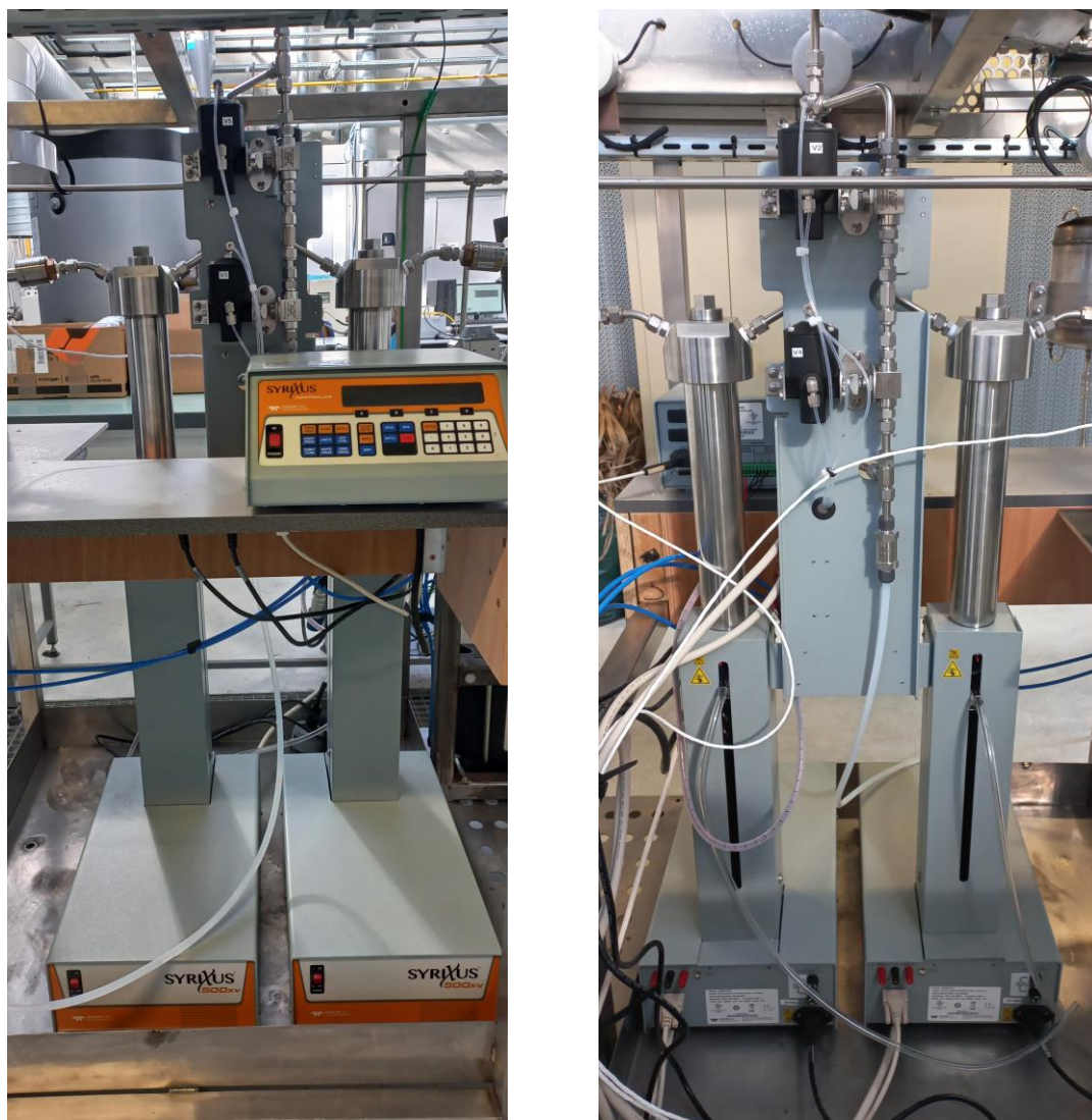
Figure 5: Recto-verso photos of the pumping system mounted on the frame of the continuous unit
