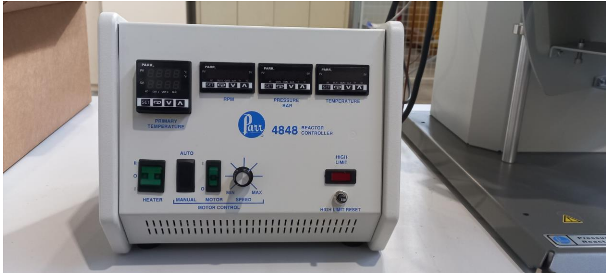
Figure 8: CSTR Reactor controller
