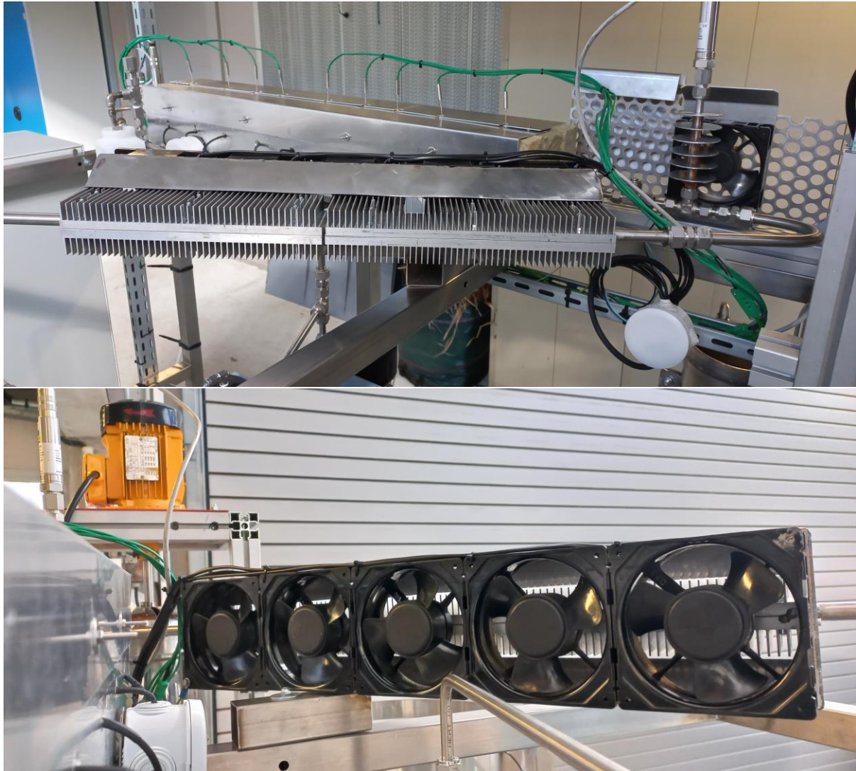
Figure 11: Front and back view of the cooling system mounted on the continuous unit's frame
