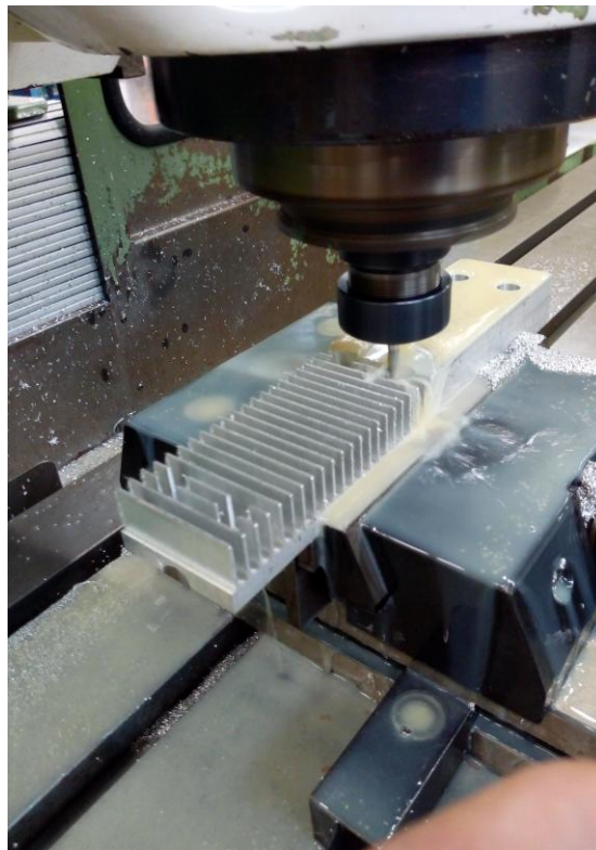
Figure 10: Fins casing manufacturing for the cooling system
