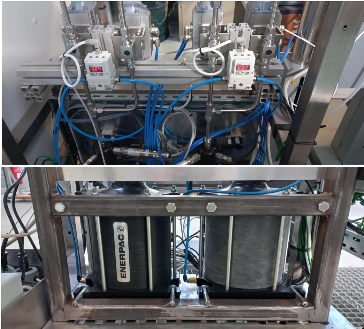
Figure 13: Pressure let-down system; air hydraulic boosters, pneumatic control valves and limit switches (front and back views)
