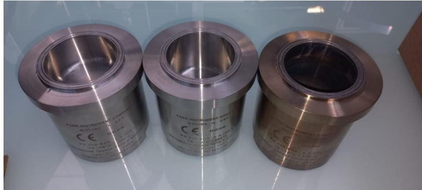
Figure 6: 100-, 150- and 250-mL reactor vessels; same outer geometry, however, the internal diameter differs to obtain the desired volume
